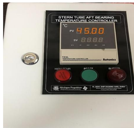
Gambar 1. Temperature Control aft bearing kapal MT. Kuang
